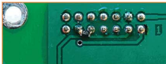
Figure 4. This resistor tells the firmware that the circuit has been modified as shown in Figures 1, 2 and 3.
